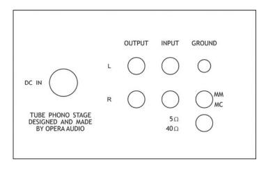
From left to right: Interconnect power cords, Output RCA jacks.(red /black ), Input RCA jacks, Grounding jack And MM / MC switch, Gain switch.
