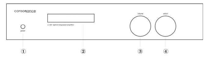
The amplifier is switched on with the button ①② Display. By pushing the same button one more time the power is switched off.
